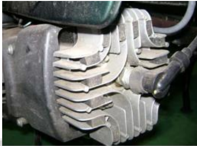
Figure 1. Engine cylinder head with rubber dampers (black color) between the fins [5]
